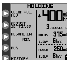
Figure 18B. HOLDING mode options, intermittent feeding mode.
